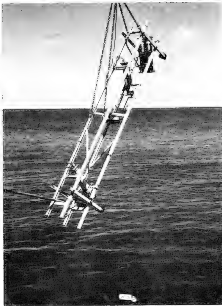
Fig. 6. A bottom-photography equipment as used on the R.V. Chain by the Woods Hole Oceanographic Institution. Two cameras at the top produce a stereo pair of photographs. A 100 w.s. strobe is at the bottom. The "pinger" is located at the center.
